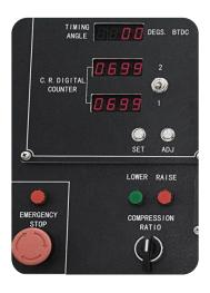
The C.R. Digital Counter and Ignition Timing Values are displayed directly on the control panel for easy reference and recording.
