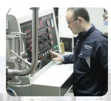
**FTC-M2 Octane Engine** – a standardized single cylinder, four-stroke, variable compression ratio, carbureted engine runs octane rating in accordance with a defined set of operating conditions in ASTM D2699 & ASTM D2700.
