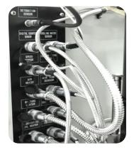
**All The Sensors Assemblies** are safely, securely and easily connected to the control unit through waterproof aviation connectors.
