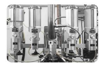
**The Four-Bowl Carburetor** is available in a variety of jet and venturi sizes for a wide range of applications. A fuel flow control system is used to adjust the fuel-air ratio. The fuel level range to produce maximum Knock Intensity is 0.7 in. to 1.7 in. The carburetor is equipped with a cooling system connected to the air control unit.
